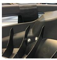
Align the #4 strap on the rear of the rear seat. Using strap, mark holes where drilling is needed. Drill holes, attach rivets and repeat for opposite side.
