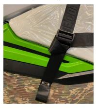
Align ends that will be riveted (under plastic trim) with the colored plastic trim on each side.
