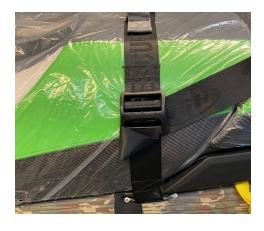
Align the #3 strap (with handle) on the rear of the front seat. Level bracket, using bracket mark holes where drilling is needed. Drill holes, attach rivets and repeat for opposite side.
